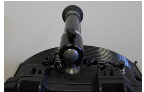
Figure 3.1.c – pivot screw controls swivel of monitor.
