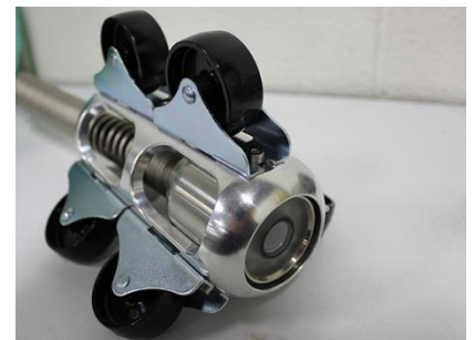
Figure 6.3.1.a – KK55 Roller Skid with larger wheels
